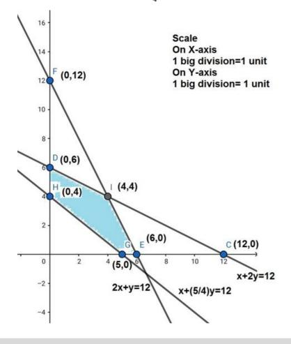
Thus the maximum profit is of Rs 40 obtained when 4 units each of item A and B are manufactured.
